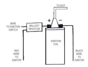
Figure 2 - Wiring Diagram
