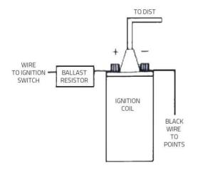
**Figure 1** - Wiring Diagram
