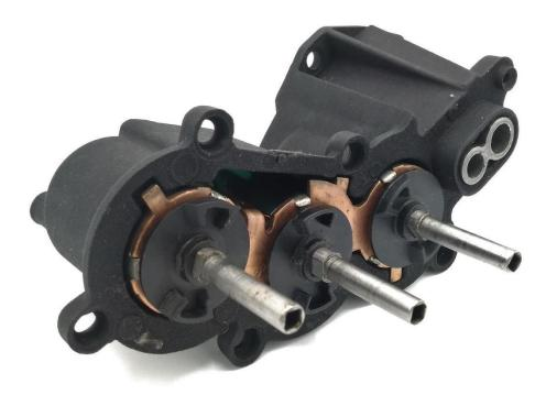
Figure 6: Solenoid block within the bigger half of the seat gear box casing
