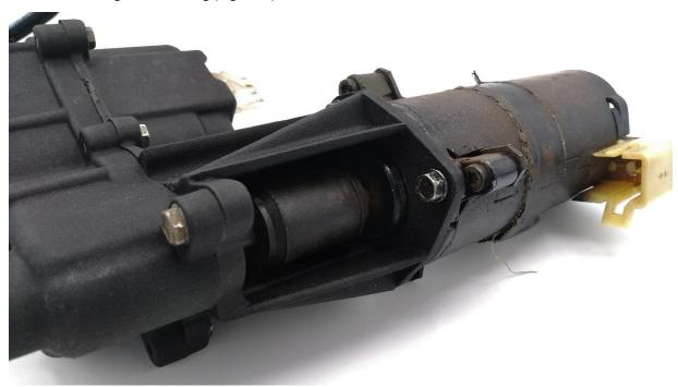
Figure 9: Assembled gearbox casing and motor
