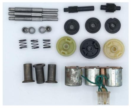
Figure 3: Seat Gearbox internal components
