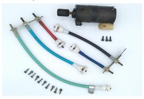
Figure 2: Seat Gearbox external components
