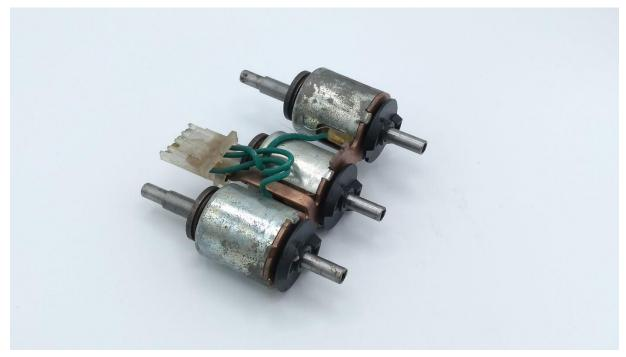
Figure 5: Solenoid block with drive shafts and plastic clutches added
