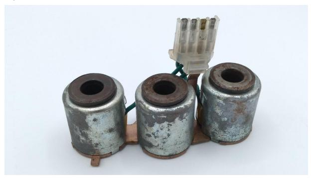
Figure 4: Solenoids with sleeves inserted.
