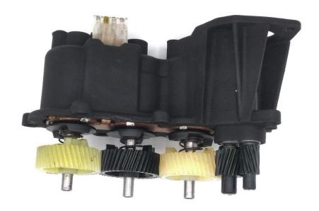
Figure 7: Assembled solenoid block with gears and springs fitted
