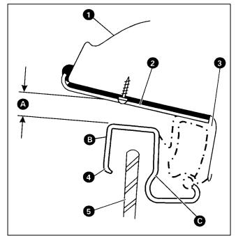
Fig. 1 Section through door and aperture
