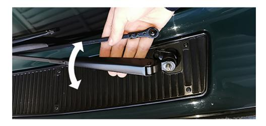
Manoeuvre and, once loose, remove the arm from the spindle.
