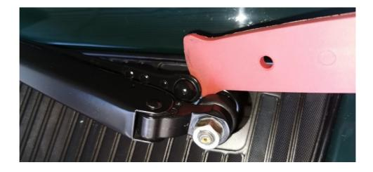
5) Remove the M4 pinch bolt (CD6839). If corroded, replace.
