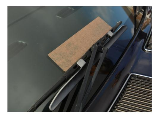
4) On the driver's side, lever the support linkage from the spindle base/ball pin using the plastic tool shown below. Some force may be necessary to remove the support arm from the ball pin, but DO NOT USE ANY METAL TOOLS HERE, as otherwise you WILL scratch surrounding paint surfaces.
