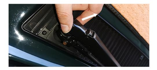
3) Ensure the wipers are fully parked. Mark the position of the blade on the windscreen using adhesive tape as below.
