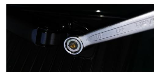
Undo the nut (driver's and passenger's side)
