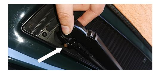
6) Undo the nuts on both sides and remove the wiper arms from the spindles. The original locking paint and/or corrosion can cause the wiper arms to stick on the spindles. DO NOT USE ANY TOOLS TO EASE THEIR REMOVAL. Carefully manoeuvre the arm back and forth to loosen them and lift off.
