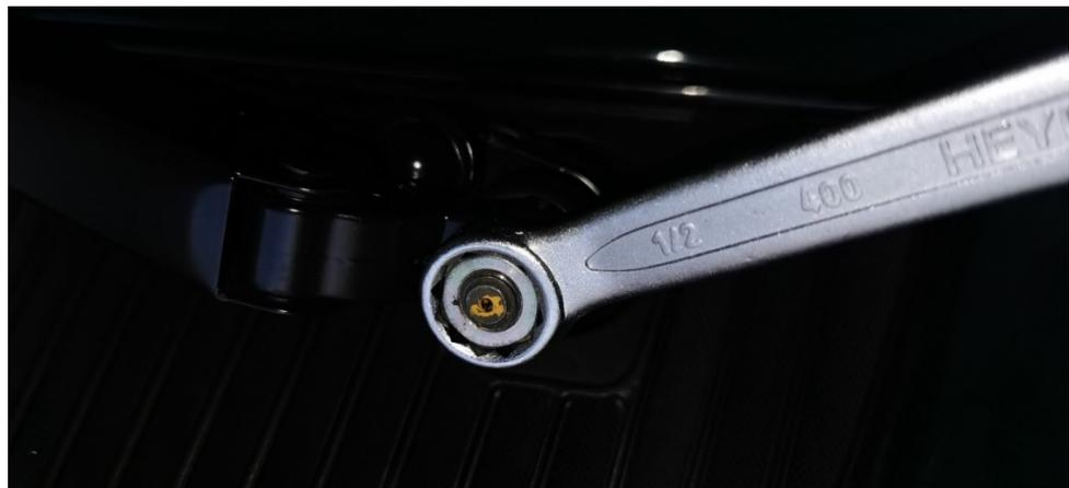
Undo the nut (driver's and passenger's side)
