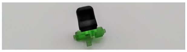
Figure 10: Rocker switch attached with superglue to the new toggle insert
