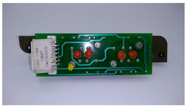
Figure 6: Backside of the switch, showing the screw nuts and screw locking glue
