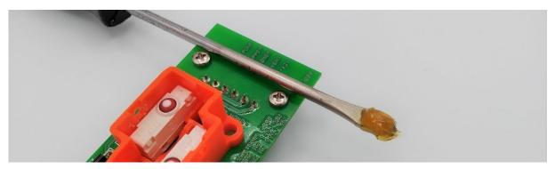
Figure 13: Amount of grease to be applied beneath the toggle case onto the pin
