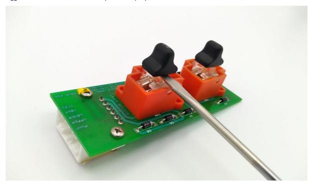
Figure 7: Position of how the slotted screwdriver shell be placed below the rocker switch
