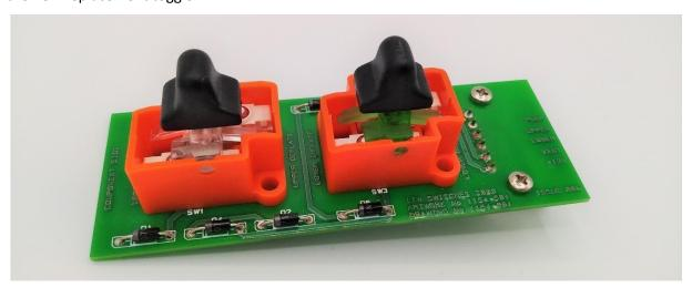
Figure 14: Assembled switch panel with the new replacement toggle insert
