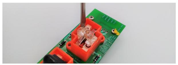
Figure 11: How to position the slotted screwdriver for removal and fitting of the toggle insert. Turn it to widen the case to release the toggle.
