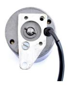
8) Fit the motor & plate assembly to the gearbox, rotating the worm drive so that the nylon coupling engages fully with the pin on the motor shaft.
