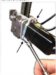
2) Remove the original adaptor plate by undoing the slotted screw and allen screw. Discard the slotted screw and plate, but retain the allen screw for later use:
