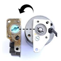
9) Now, re-using the allen screws retained in no. (4) above, fit the motor and plate assembly to the gearbox, as in (A) & (B) below. Please note: if the gearbox is equipped with a UNF thread in position (B), re-use the allen screw retained in instruction no. (2).
