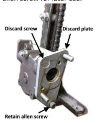
3) If your new motor is supplied with this teardrop-shaped adaptor plate, remove and discard it (it is used on pre-Bosch type window lift motors only):
